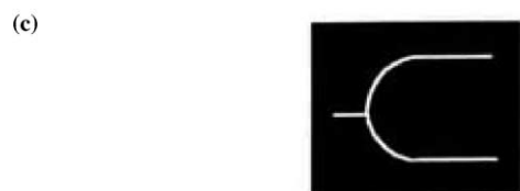
Fig. 5. The perpendicular disclinations of \chi @ \lambda^- + \tau^+ (i.e. \lambda^- \tau^+ ). (a) SEM photograph of this disclination pairs; (b) schematic structure of this disclination pairs (the dashes represent the directors parallel to the paper plane, while the dots represent the directors perpendicular to the paper plane); (c) schematic picture shown in SEM photograph.
