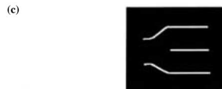
Fig. 6. The perpendicular disclinations of \chi @ \tau^- + \lambda^+ (i.e. \tau^- \lambda^+ ). (a) SEM photograph of this disclination pairs; (b) schematic structure of this disclination pairs (the dashes represent the directors parallel to the paper plane, while the dots represent the directors perpendicular to the paper plane); (c) schematic picture shown in SEM photograph.
